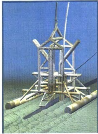
TRENCHING JET SLED
